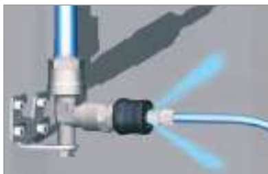
El aire es expulsado completamente Air is exhausting completely
